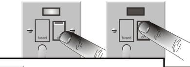
3. Switch it back on. The light on the heater should be flashing; if it is not flashing restart the procedure.
