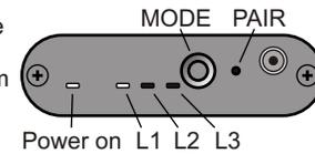
PAIR is pressed with the supplied pin during system setup.
